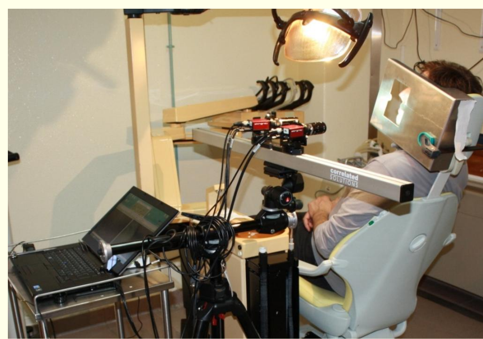
Fig 3. 3D Digital Image Correlation system set up (Correlated Solutions®, Columbia, USA).
