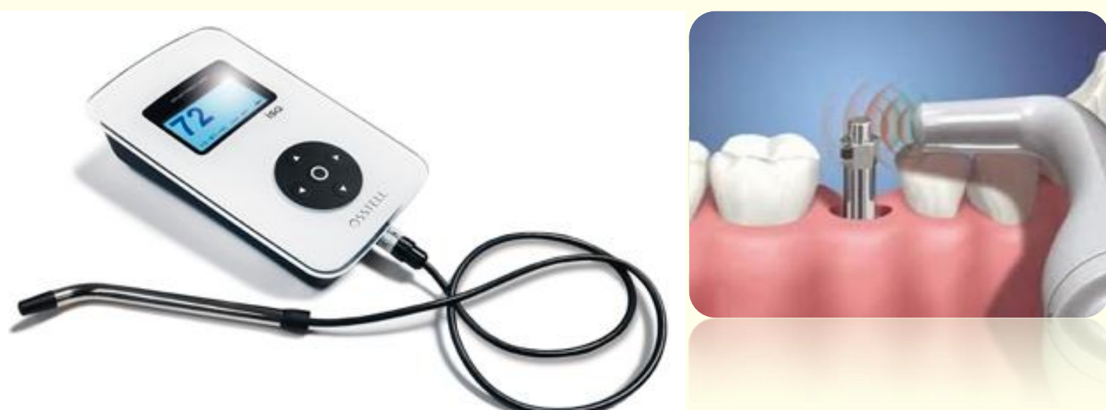
Fig 5. Ostell® ISQ (Ostell® ISQ Integration Diagnostic, Sweden) used in this study to assess implant stability, and diagram image of device functioning.
