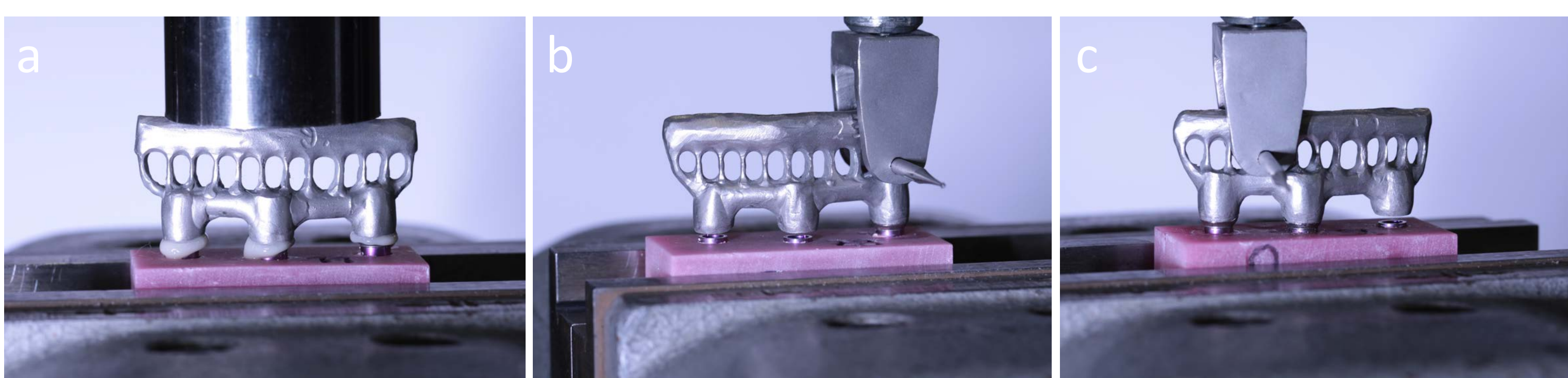
Fig. 3: (a) Standardized cementation of the frameworks with a 5kg load for 10 min for each cement (here example of cementing all 3 "crowns"). (b) Pulling-off test by using a universal testing machine (Zwick®): here simulation of a single crown removal. Pulling-off approach directly on the top of one implant. (c) Removal of a framework simulating a situation of two splinted crowns. Pulling-off approach between two neighboring implants.
