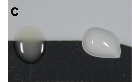
**a**:The translucent adhesive cement; **b**:The opaque adhesive cement with the accompanying silane coupling agent; **c**:Visual evidence of the different translucencies of both cements.
