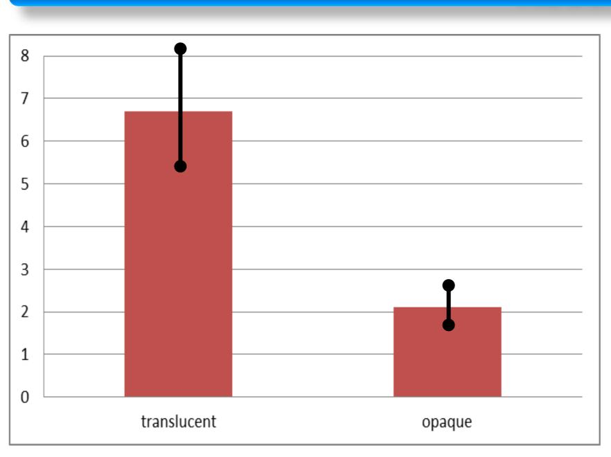
The final color of the abutment crowns were significantly affected by the translucency of both tested adhesive cements. M cement resulted in a  $\Delta E$  value of 6.7±1.9 (P<0.05) . Cement M resulted in less color difference than P (P<0.05); that had a  $\Delta E$  value of 2.1±0.6.
