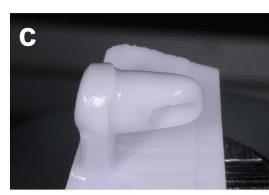
**a**:Digital design of the abutments; **b**:Lithium disilicate abutment block, **c**:The milled abutment before crystallization phase (after screw detachment, the abutments were crystallized according to manufacturers' instructions).
