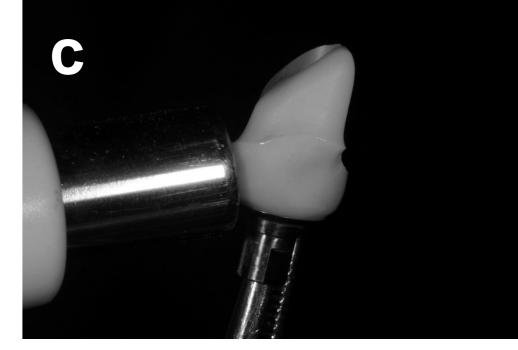
a:Reference sample for CIE Lab measurements; **b**:Reference measurements from the sample with a contact type dental spectrophotometer; **c**:Colour measurements from the abutment. Both calculations were repeated 3 times and then their median values were obtained and  $\Delta E$  values were achieved according to CIE Lab formulae.
