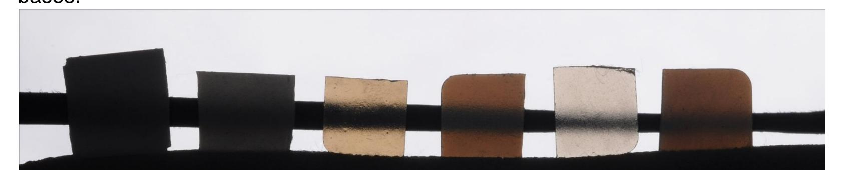
When 0.5 mm slices are obtained from zirconia and lithium disilicate (E) materials, zirconia appears opaque while glass-ceramic materials bear varying degrees of translucency that helps mimicking natural esthetics. (Left to right: zirconia, E-high opacity, E-medium opacity, E-low translucency, E- high translucency, leucite ceramic)
